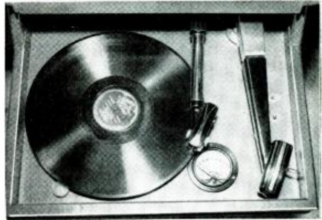
Motorboard holds two pickups, one for good discs, one for bad.
