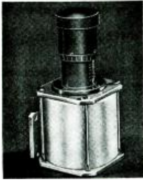
Fig. 13—Cavity wavemeter for 8400-9800 mc.
