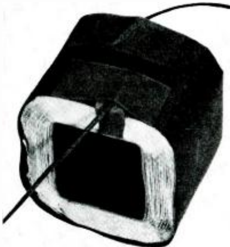
Adhesive strips make external connections stronger. Whole winding may be taped also.
