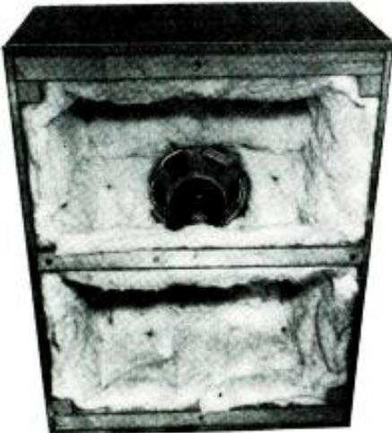
Fig. 3—Inside of speaker cabinet is padded.
