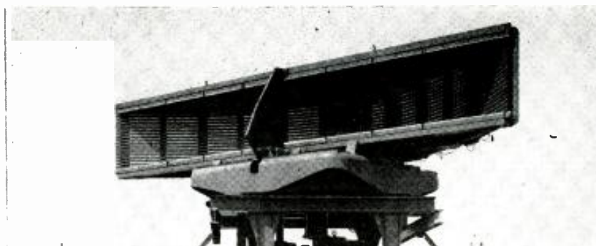
Close-up of the rotating "cheese" antenna, built of strips to reduce wind resistance.
