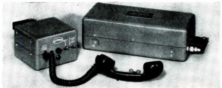
Raytheon transmitter-receiver (right) and control box (left) show compactness of equipment.
